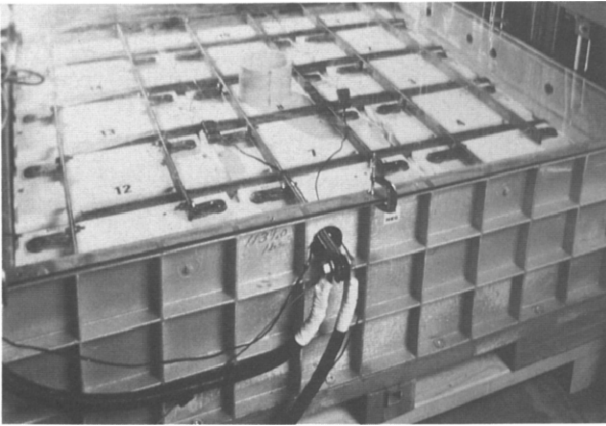
Fig. 10. View of a JCI module inner assembly of 15 parallel batteries, under test at Argonne National Laboratory.
